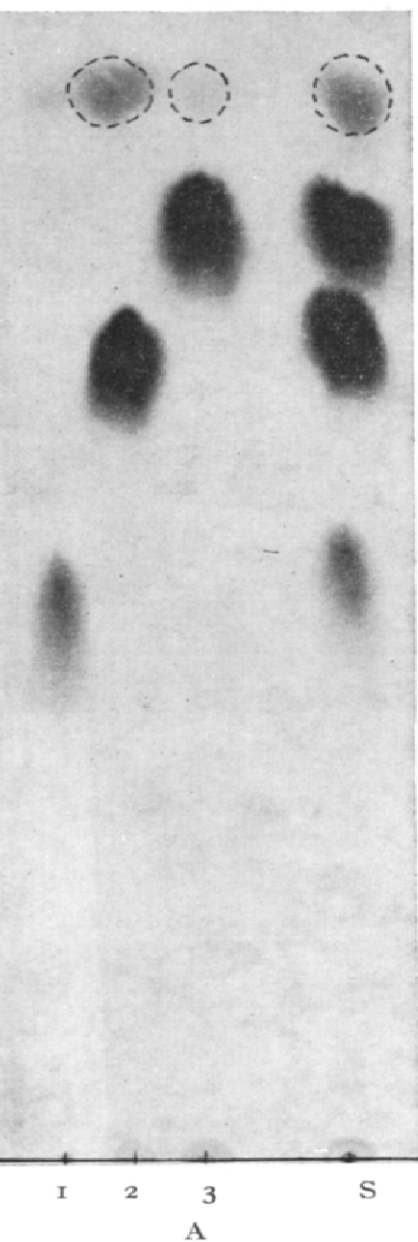
Fig. 3. Example of a chromatographic separation of a mixture of solubilized vat dyes. A. Descending technique. B. Centrifugal technique. 1 = Indigosol O6B; 2 = Indigosol Orange HR; 3 = Anthrasol Pink IR; S = mixture of 1, 2 and 3.
